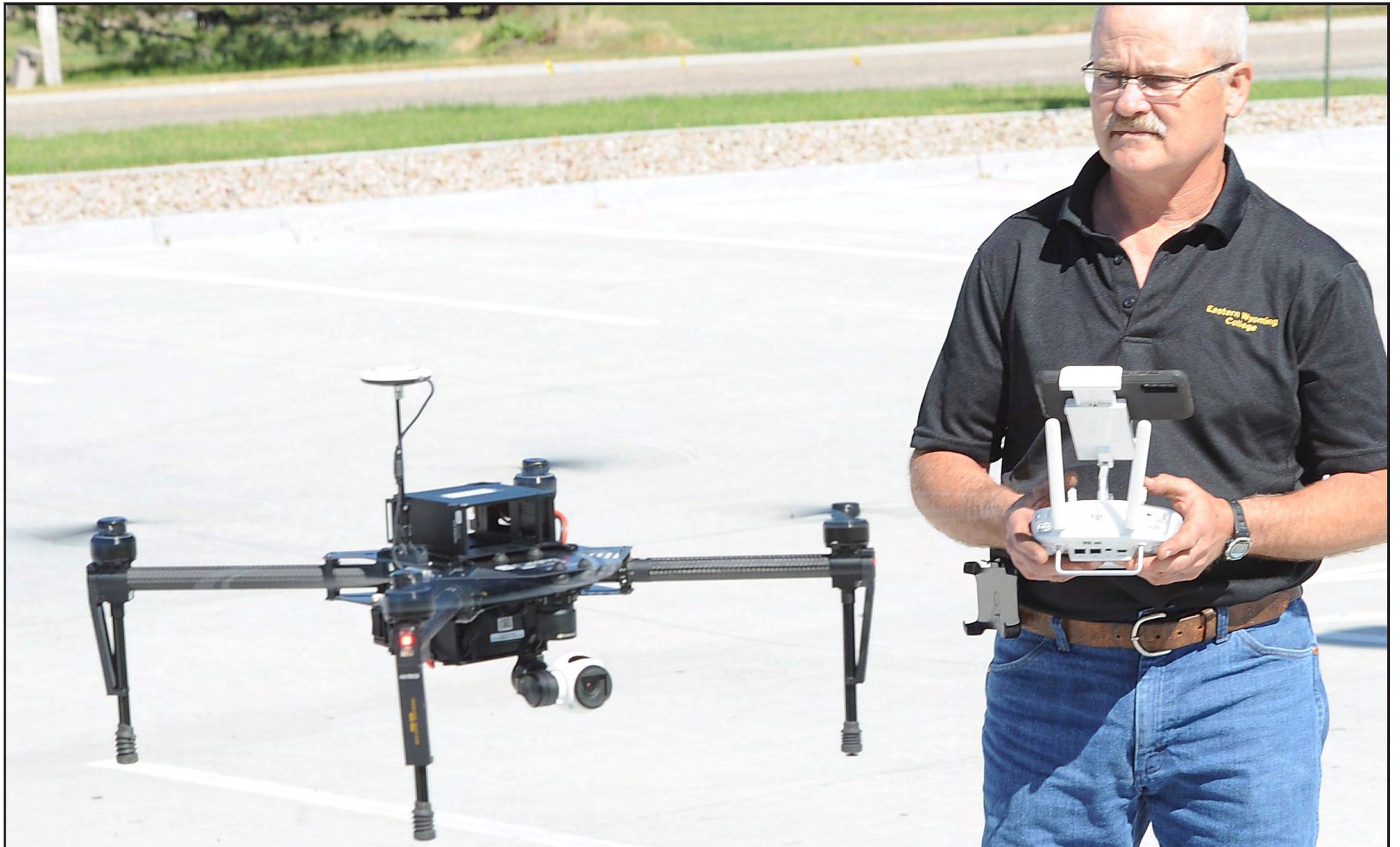
Eastern Wyoming College professor Matt Scott flies a DJI Matrice 100 drone. It has an expandable platform drone that can have different payloads or sensors added to it to increase its versatility. Drone on the EWC campus. Drones allow for more detailed data making the decisions needed for those working in the field of precision agriculture. For more information on the program contact Scott at msscott@ewc.wy.edu .
